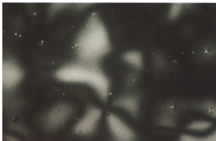
Figure 3. Liquid crystal textures of EPTB-CDA10 observed by Polarized Microscope at 70 °C. (Magnification : \times 100 )
